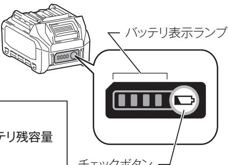
The diagram shows a side view of a power tool with a battery pack attached. A callout box points to the 'Battery Indicator Lamp' (バッテリ表示ランプ) on the front of the battery, which is a row of seven rectangular lights. Another callout box points to the 'Check Button' (チェックボタン) located below the indicator lamp.
